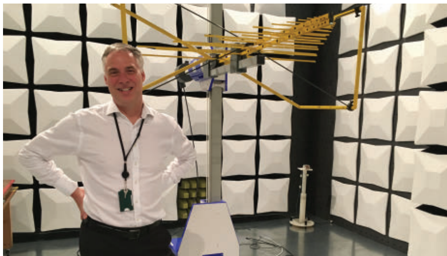
RFI experts at Curtiss-Wright Defense Solutions use an anechoic chamber to determine some of the best ways of mitigating unwanted RF energy.
