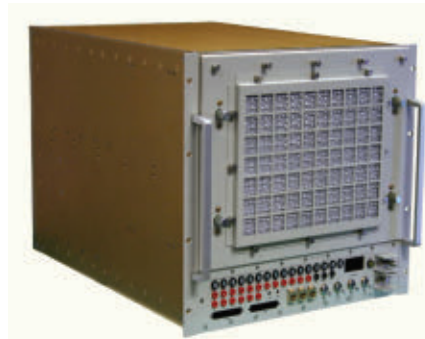
A honeycomb filter sits on the exterior of an Elma Electronics system and helps reduce EMI/RFI through the individual cells, which reflect and absorb noise.
