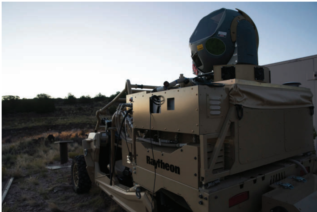
Fast-moving laser weapons like this prototype mounted to a light tactical military vehicle depend on reducing component size, weight, and power consumption (SWaP).
